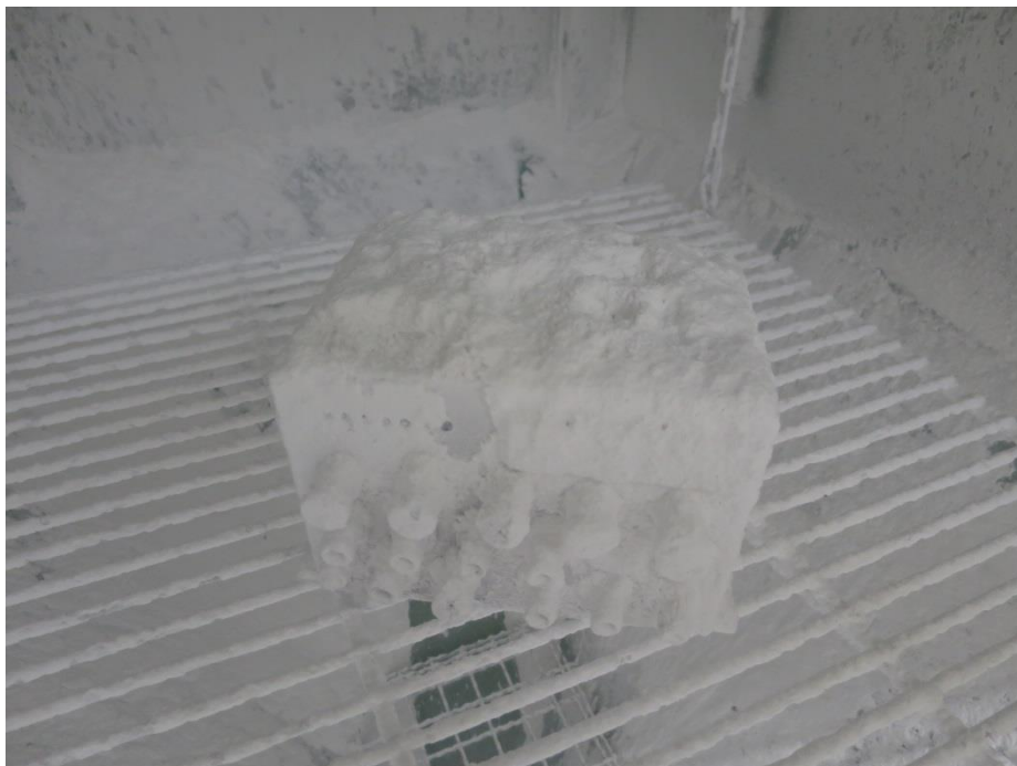
Arrangement of device under test in the dust chamber after the dust test
