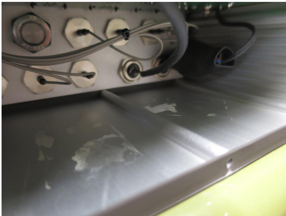
Open Housing: No dust penetrated
