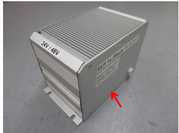
Device under test 01 Overview Rear (Arrow: Hole for under pressure connection)
