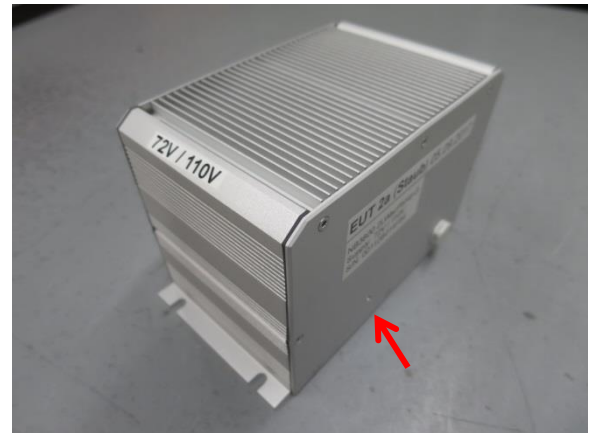
Device under test 03 Overview Rear (Arrow: Hole for under pressure connection)
