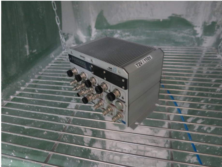
Arrangement of device under test in the dust chamber before the dust test
